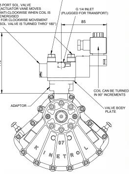
Single solenoid, 3 or 5 port, interchangeable for double acting or spring return, NAMUR interface. Most brands of NAMUR interface solenoid valve can be supplied to special order.
